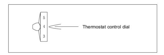
The marks on the knob are the temperature grades, not the exact number of the degrees of temperature."0" shows a forced STOP and "7" shows the lowest temperature.
